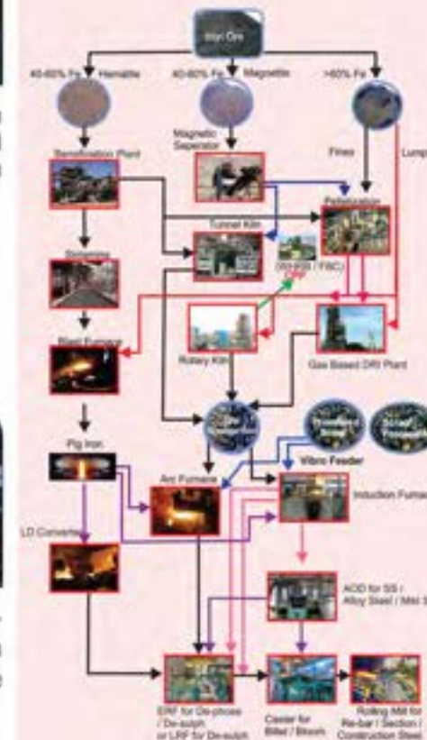
ERF® (Electrotherm Refining Furnace) with ELdFOS® technology, a special metallurgical equipment for carrying out de-phosphorization and de-sulphurization in the same equipment.
