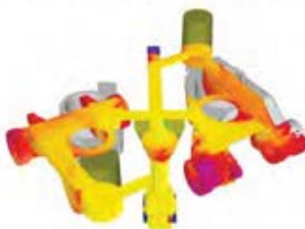
From Unrigged Casting to Fully Rigged Model
