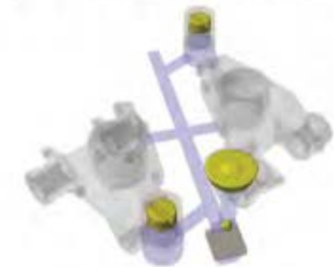
CFD Analysis and Shrinkage Prediction
