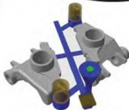
From Unrigged Casting to Fully Rigged Model
