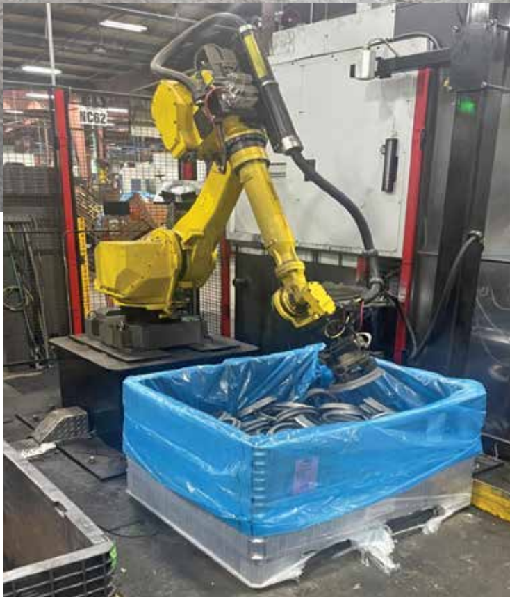
Heishman explained robotic bin picking with machine vision.
