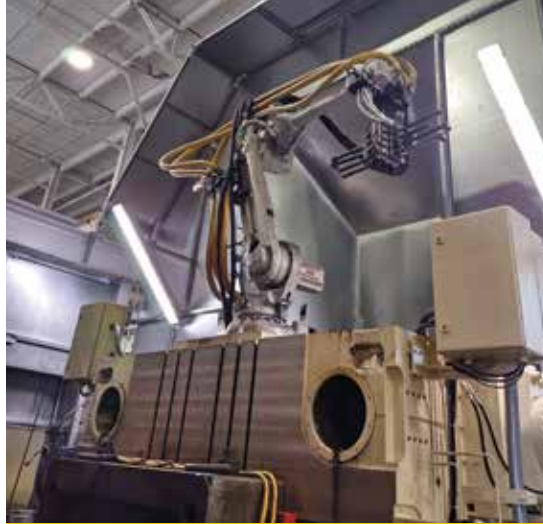
This robot is used for spraying die halves of the mold with lube to help take the parts out of the mold after casting. The foundry collects data points for die lube pressure and volume being used to ensure its process is the same every time the robot runs through its cycle.
