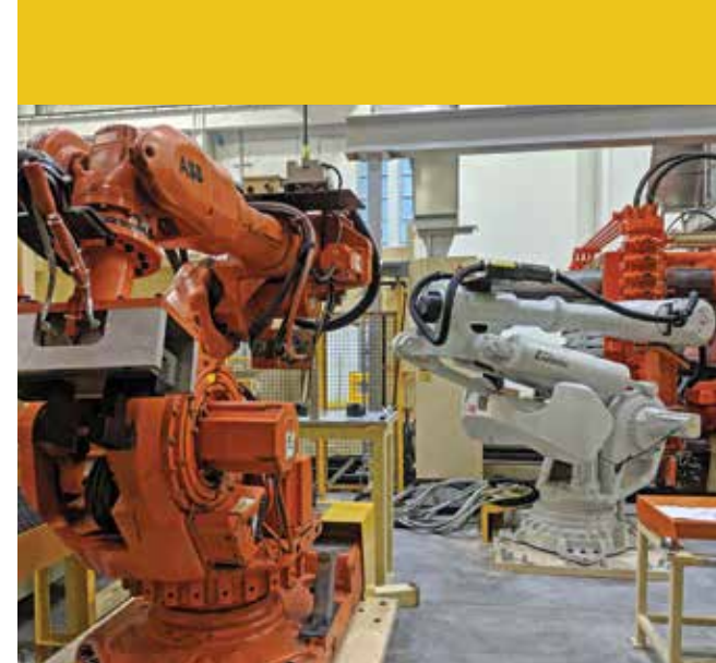
Two robots are in this diecasting cell—one is an extraction robot that pulls the casting from the die; the other is a process robot that assists with loading the casting for sawing, laser marking, and other processing. Mercury Marine connects to robots to get signals to help understand the process and the cycle times associated with robot movements.
