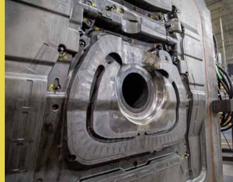
A central gating system in the mold directs the liquid metal into and throughout the cavity so the entire casting is filled with metal before solidification. This avoids leaving pockets of space within the part that would make it defective.
