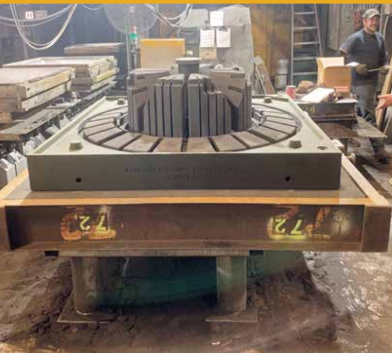
University of Northern Iowa produced the heavy and intricate 3D-printed sand mold. It then traveled six-and-a-half hours northwest to Dakota Foundry located in the northeastern part of South Dakota.
