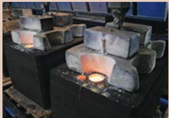
The bronze alloy for DeVore's castings contains copper and tin, according to Bryan Greene, operations manager at Ball Brass, making for a good finish. "It's easy to grind, and after polishing, it creates a nice patina on the casting," he said.
