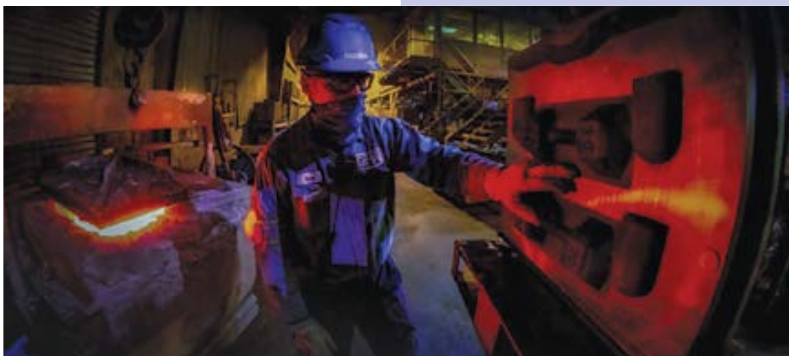
A GLC worker inspects the pattern used for the molds for the handweights.
