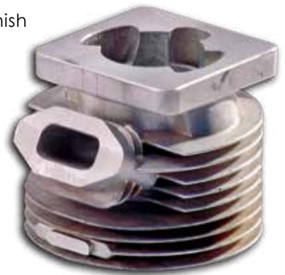
PreciseCast Prototypes & Engineering was able to 3D print a wax corebox to produce a single plaster core.
