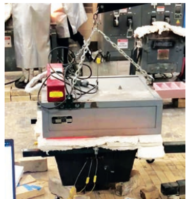
Left: A steel beam instrumented with four strain gauges. Right: A box furnace is lifted before molten steel is poured into a container embedded with fiber optic sensors.
