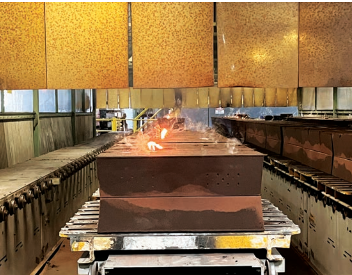
A simmering mold containing molten metal gets a time out to cool off.
