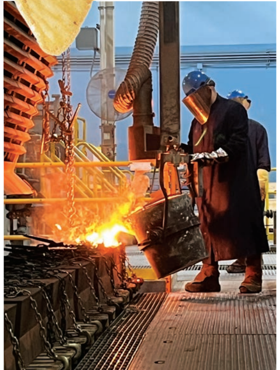
A foundry operator in full protective gear pours melted metal into molds to make castings.
