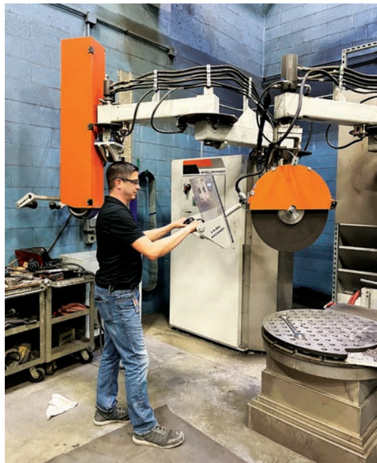
Foundry Supervisor Travis Rogriguez demonstrates a robotic saw for cutting loose ends off castings.
