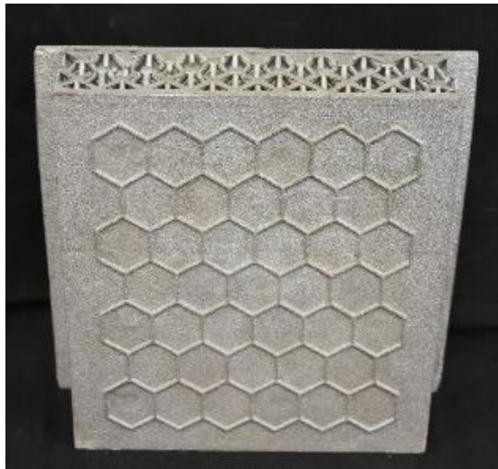
Complex lattice casting produced by Eck Industries in A206 alloy reinforced with 1% TiC nanoparticles
