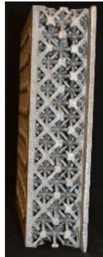
Complex lattice casting produced by Eck Industries in A206 alloy reinforced with 1% TiC nanoparticles
